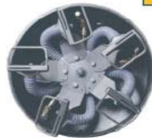
The five vacuum heads and three spray jets rotate at 130 RPM creating 650 complete clearing passes per minute.
