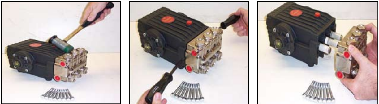
Figure 5-6. Separate Manifold from Crankcase
