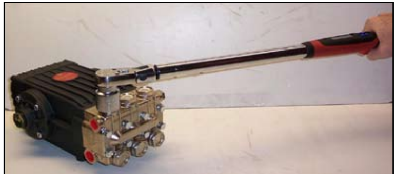
Figure 5-5. Replace Valve Cap and Torque to 95 ft. lbs. (13 m kgs)
